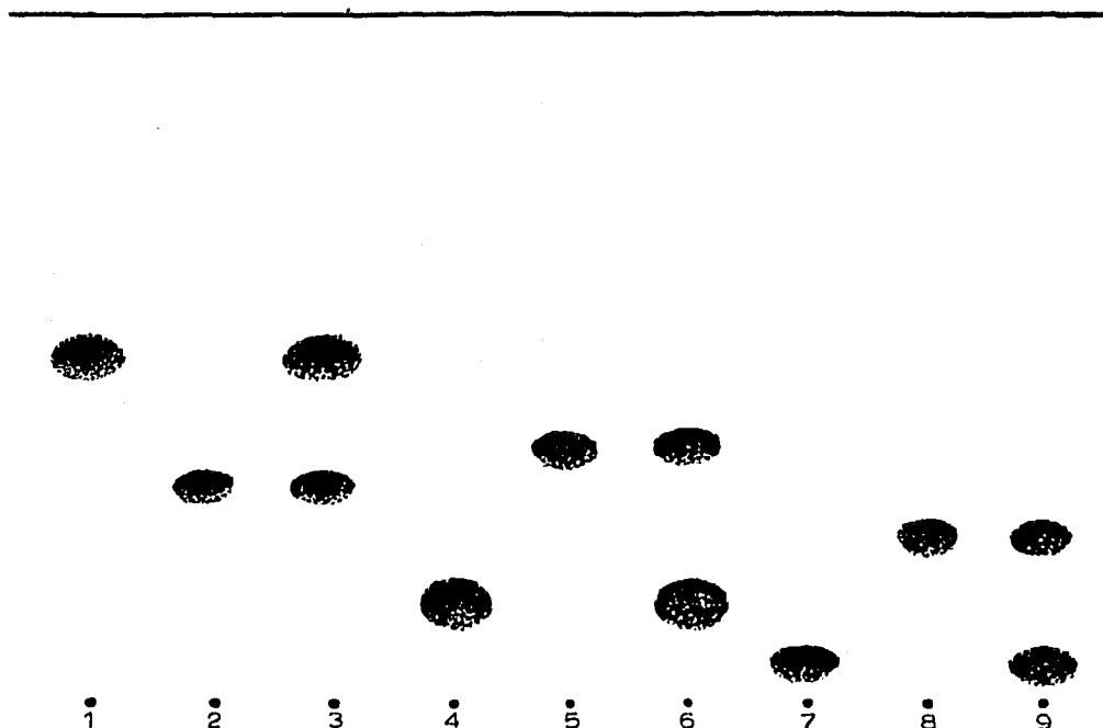
Fig. 1. Thin layer chromatogram of isomeric oximes. The oximes were dissolved in tetrahydrofuran and 10 \mu l of a 0.5% (w/v) solution of each oxime was applied to the plate. Adsorbent: silica gel G (according to STAHL). Solvent system: benzene-ethyl acetate (50:10 v/v). Solvent front 14 cm. Spraying reagent: saturated alcoholic solution of cupric acetate monohydrate. (1) \alpha -Benzaldoxime; (2) \beta -Benzaldoxime; (3) Mixture of isomeric benzaldoximes; (4) \alpha -Benzoin oxime; (5) \beta -Benzoin oxime; (6) Mixture of isomeric benzoin oximes; (7) \alpha -Anisoin oxime; (8) \beta -Anisoin oxime; (9) Mixture of isomeric anisoin oximes.
